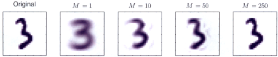
Figure 12.5 An original example from the off-line digits data set together with its PCA reconstructions obtained by retaining M principal components for various values of M . As M increases the reconstruction becomes more accurate and would become perfect when M = D = 28 \times 28 = 784 .
