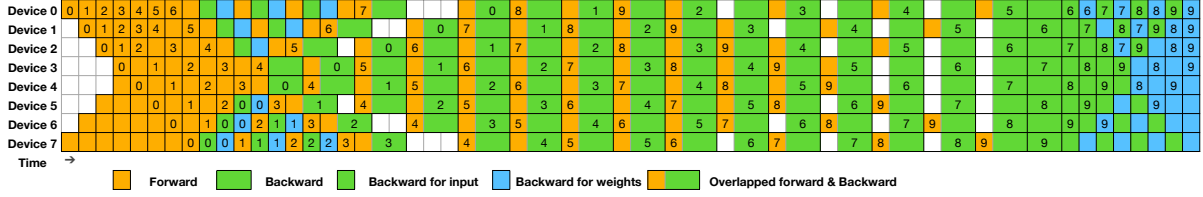
Figure 5 | Example DualPipe scheduling for 8 PP ranks and 20 micro-batches in two directions. The micro-batches in the reverse direction are symmetric to those in the forward direction, so we omit their batch ID for illustration simplicity. Two cells enclosed by a shared black border have mutually overlapped computation and communication.
